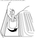
**3** Remove upper burr by rotating counterclockwise, aligning the orange arrow on the burr grinder with the orange arrow labeled ALIGN on the machine. Once aligned, lift upper burr out.
