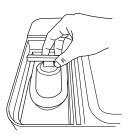
**NOTE: DO NOT** put any water in the grinder. If water does get in the grinder, please call us at 1-877-646-5288 immediately.
