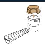
Place funnel on portafilter with double basket\*, aligning the notches on the funnel with the notches on the portafilter. Push down until funnel locks into place in the portafilter.
