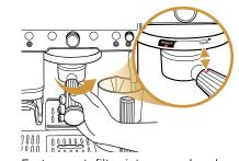
Fasten portafilter into group head until orange dot on portafilter aligns with lock arrow on group
