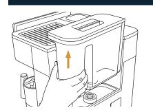
Remove water reservoir from back of machine.
