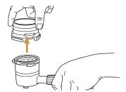
Remove funnel from portafilter. Place funnel and tamper in storage on left side of machine.
