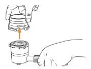
Remove funnel from portafilter. Place funnel and tamper in storage on left side of machine.
