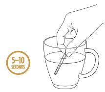
Locate test strip provided in starter kit. Completely submerge test strip in the water you plan on using with your machine for 5-10 seconds, ensuring all squares are underwater.
