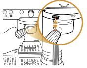
Place portafilter in group head (angled to the left) by aligning orange dot on portafilter with orange dot on group head.
