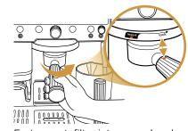
Fasten portafilter into group head until orange dot on portafilter aligns with lock arrow on group
