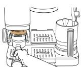
With the funnel on top of the portafilter, insert portafilter in the grinding cradle. Make sure it is level and fits securely. Once portafilter is installed in grinding cradle, it will be weighed. To ensure accurate weight, let go of portafilter.
