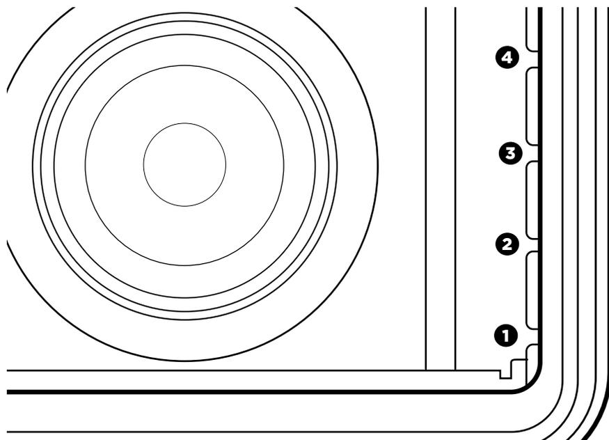
The oven has 4 available rack positions where your accessories can slide into the unit (**see image above**). When you select a function, the corresponding rack number(s) will illuminate on the control panel. The numbers on the control panel (**see Fig. 1**) will coincide with those on the interior of the unit. See the chart on page 8 for further details.
