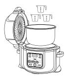
2 Assemble the pressure lid by aligning the arrow on the front of the lid with the arrow on the front of the cooker base. Then turn the lid clockwise until it locks into place.
