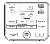
**NOTE:** If running for 1 hour or less, the clock will count down by minutes and seconds. If running for more than 1 hour, the clock will count down by minutes only.
