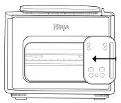
You can open or close the door when the SmartSwitch is in either the COMBI COOKER or AIR FRY/STOVETOP position.
