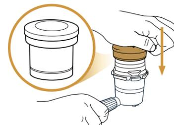
After grinding, remove portafilter. On a solid level surface with funnel still attached, **press tamper all the way down until it meets funnel.**
