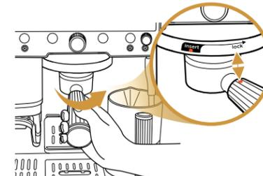
Fasten portafilter into group head until orange dot on portafilter aligns with lock arrow on group head.
