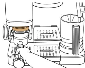
With the funnel on top of the portafilter, insert portafilter in the grinding cradle. Make sure it is level and fits securely. Once portafilter is installed in grinding cradle, it will be weighed. To ensure accurate weight, let go of portafilter.
