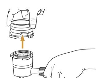
Remove funnel from portafilter. Place funnel and tamper in storage on left side of machine.
