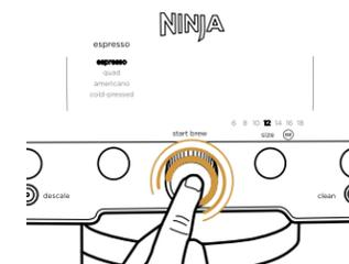
Press **START BREW**. The machine will beep to signal the brew has started. The progress bar will illuminate, indicating the status of the brew.
