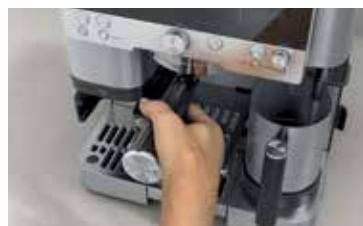
Tamp the grounds. Press tamper all the way down until it meets the funnel. Then remove funnel and install portafilter into group head by aligning orange dots and twisting to the right.
