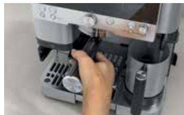
Remove funnel and install portafilter into group head by aligning orange dots and twisting to the right.
