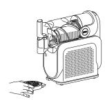
**6.** Insert the drip tray in front of the motor base until it clicks into place.
