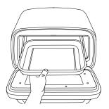
**Bake Pan:** Before placing the bake pan, ensure the pizza stone is clean and properly positioned within the grooves. Then, set the bake pan on top of the pizza stone.
