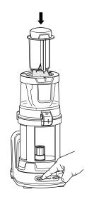
4 Select START/STOP to begin spiralizing. Continue to press firmly with Food Pusher to guide ingredient through Feed Chute.
