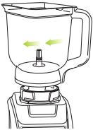
1. Place the Blender Pitcher on the base and turn clockwise to lock in place.
