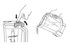
8b For thicker mixtures that cannot be emptied through the pour spout, remove the lid and Stacked Blade Assembly before pouring. To remove the lid, press the RELEASE button and lift the handle. To remove the blade assembly, carefully grasp it by the top of the shaft and pull straight up. The pitcher can then be emptied.
