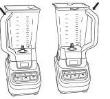
5 The pitcher can be placed on the motor base two ways; the handle can be on the front right corner or the front left corner. 6 Holding the Stacked Blade Assembly by the top of the shaft, place it onto the drive gear inside the pitcher. Ensure the Stacked Blade Assembly is seated properly and is standing upright.
