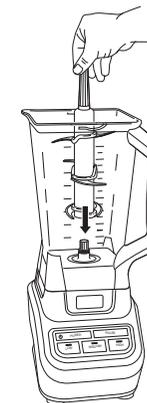
**NOTE:** The Stacked Blade Assembly will fit loosely on the drive gear.
