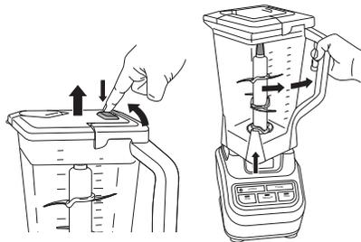
**12** To remove the lid, press the release button on the lid, pull the lid handle up to a 90° angle, and lift the lid off. Turn the pitcher counterclockwise and then lift off the base.
