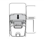
6 Center the carafe with the brew-through lid installed below the brew basket. With everything securely in place, the Drip Stop set to open, and the brewer powered on, turn the dial to select the Full Carafe size and press the BREW STYLE button to select Classic.
