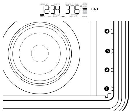
The oven has 4 available rack positions where your accessories can slide into the unit (see image above). When you select a function, the corresponding rack number(s) will illuminate on the control panel. The numbers on the control panel (see Fig. 1) will coincide with those on the interior of the unit. See the chart on page 8 for further details.
