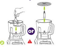
Place the desired blade or disc spindle and disc into the bowl.
