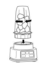
**4** Turn the cup upside down and install on the motor base by aligning the tabs on the cup with the slots on the base. Then, rotate cup clockwise until it clicks. Once locked in place, the programs will illuminate and the unit will be ready for use.
