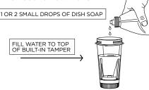
Fill with warm water up to top of built-in tamper and add 1 or 2 small drops dish soap. Install blade assembly.
