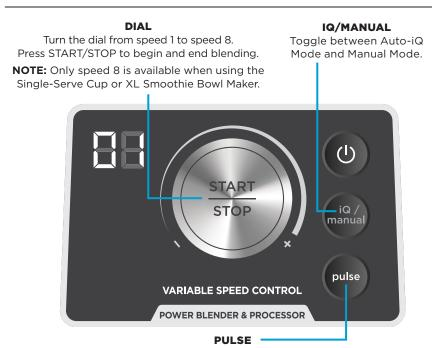
Use short presses for short pulses and long presses for long pulses.
