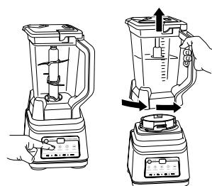
**6a** If using an Auto-iQ® program, first select the program that best suits your recipe. The preset feature will automatically stop at the end of the program. To stop the unit at any time, press the currently active button again.
