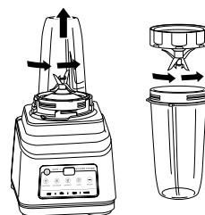
**6** To remove the cup from the motor base, turn the cup counterclockwise and then lift up.
