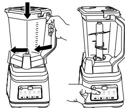
**3** Exercising care, grasp the Stacked Blade Assembly by the top of the shaft and place it onto the drive gear inside the pitcher. Note that the blade assembly will fit loosely onto the drive gear.
