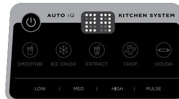
**LOW, MEDIUM, and HIGH:** When selected, each of these speeds runs continuously for 60 seconds. Press the currently active button again to stop the program sooner. They do not work in conjunction with any Auto-iQ programs.
