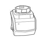
1 Plug in motor base and place on a clean, dry, level surface such as a countertop or table.
