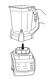
2 Lower the pitcher onto the motor base, positioning it in a diamond position, with the LOCK symbols visible on the motor base.
