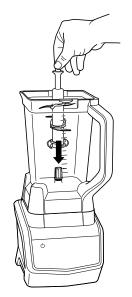
4 Exercising care, grasp the Stacked Blade Assembly by the top of the shaft and place it onto the drive gear inside the pitcher.
