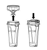
8 Turn cup over so blade assembly is on top. Rotate blade assembly counterclockwise to remove. To take your blended contents on the go, place the sealed spout lid on cup and turn clockwise to seal.
