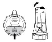
7 With cup flat on the counter (with blade assembly on the bottom), pull up on the vacuum release tab. Once the vacuum is released, you'll be able to remove the blade assembly.
