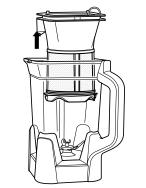
**11** Unplug the unit when finished. To lift motor base, place your hands underneath both sides of it and gently pull the unit up and toward you.
