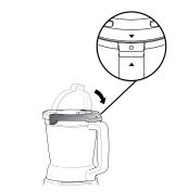
4 Place the lid on the bowl, aligning the triangle symbol on the lid with the triangle symbol on the handle. Press down on the handle until it clicks into place. Once the lid is locked in place, the available program buttons will illuminate.
