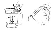
**8b** For thicker mixtures that cannot be emptied through the pour spout, remove the lid and Stacked Blade Assembly before pouring. To remove the lid, press the RELEASE button and lift the handle. To remove the blade assembly, carefully grasp it by the top of the shaft. The pitcher can then be emptied.
