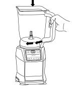
2 Lower the Total Crushing Pitcher onto the motor base. The handle should be aligned slightly to the right and the pitcher should be oriented so the **LOCK** symbols are visible on the motor base. Rotate the pitcher clockwise until it clicks into place.
