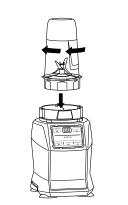
4 Turn the cup upside down and install on the motor base. Align the tabs on the cup with the slots on the base, then rotate cup clockwise until it clicks into place. Once the cup is locked in place, the available program buttons will illuminate and the unit will be ready for use.
