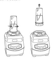
7 To remove the Nutri Ninja cup, ensure that the motor has stopped running. Then turn it counter-clockwise and pull straight up to remove.
