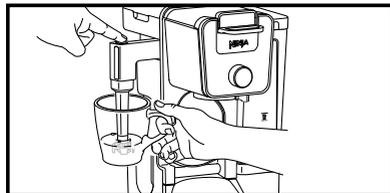
2. Swing the arm of the frother toward the front of the brewer. Install the frother whisk by twisting it to the right.
