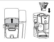
2 Ensure the adapter is in the REMOVE position before installing. Then place the adapter over the brew basket and push down firmly so it is fully seated.
