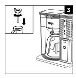
Twist the **Brew-Through Lid** clockwise onto the **Carafe** to lock into place and center the carafe below the brew basket.
