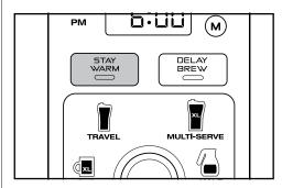
Press **STAY WARM** after the brew to turn the Intelligent Warming Plate off. To turn the Intelligent Warming Plate on at any time turn the dial to one of the carafe sizes and press **STAY WARM**.
