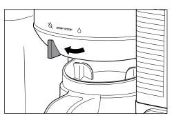
When the brew cycle is complete, set the Drip Stop to the closed position to stop dripping from the brew basket. While the Drip Stop is closed, the Drip Stop indicator will illuminate.
