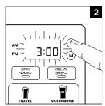
Quickly press the hour (H) and/or minute (M) buttons to increase the time up to 4 hours or decrease the time to 0 hours. Press **STAY WARM** to set the new time. The brewer will automatically save the new time after 5 seconds of inactivity.
