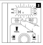
Next, the clock will display the current warming plate temperature. To keep the same temperature, press **STAY WARM**, or wait 5 seconds for the same temperature to lock in. To change the temperature, press the hour (H) or (M) buttons, then press **STAY WARM**. The brewer will automatically save the new time after 5 seconds of inactivity.
