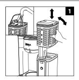
Lift the **Water Reservoir** to the right and up off the coffee maker. Flip the **Reservoir Lid** open or remove the entire lid. Add water up to, but not exceeding, the **Max Fill** line. Return the water reservoir to the coffee maker.
