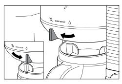
When brewing a carafe, close the **Drip Stop** to pause the brew cycle and pour a cup. Promptly replace the carafe and open the Drip Stop to complete the brew.
