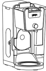
Ensure the brew basket is installed and the Ninja Pod Adapter is removed. Then, insert a paper filter in the basket (refer to steps on pages 4 and 5).
