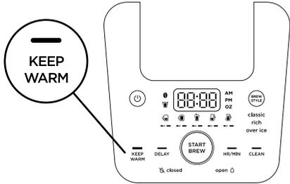
The Intelligent Warming Plate will automatically turn on while brewing a Classic or Rich brew on any Carafe size and remain on for 2 hours. To adjust how long the Intelligent Warming Plate remains on (up to 4 hours), refer to the Owner's Guide.
