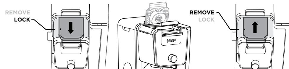
1. Once the adapter is installed in the brewer, make sure the position indicator on the left side of the adapter is aligned with LOCK by pulling the handle toward you. Then, lift to open the handle, insert a pod, firmly push down on the handle to pierce the pod, and begin programming your brew.
