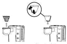
Remove the permanent filter, then fold a #4 paper cone filter along the seams. Open the top fully, then insert filter firmly into the filter holder.
