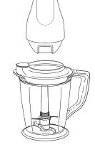
7 Place the Master Pod on top of the pitcher splash guard making sure that it is securely in place. **DO NOT** attempt to operate the appliance without the safety splash guard in place.
