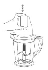
8 To start the appliance, plug the power cord into the electrical outlet, securely hold the Master Pod while operating and press on the on/off pulse button located on the top of the Master Pod 9 Hold the Master Prep® pitcher firmly while depressing the on/off pulse button to ensure the unit stays in place.
