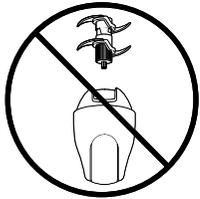
**IMPORTANT: DO NOT** try to place the Chopping Blade Assembly onto the power head and then into the Master Prep® Professional Chopping Bowl.
