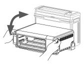
**4** Press the push button to release the back door to access the oven's interior.
