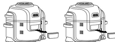
**NOTE:** Prior to each use, make sure the silicone ring is well seated in the silicone ring rack and the anti-clog cap is mounted properly on the pressure release valve.
