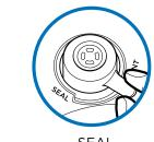
Turn Pressure Release Valve to SEAL
