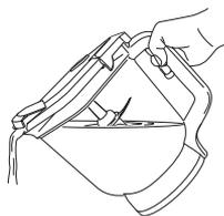
**⚠ WARNING:** Stacked Blade Assembly is sharp and not locked in place. If pouring with the lid removed, carefully remove the Stacked Blade Assembly first, holding it by the shaft. Failure to do so will result in a risk of laceration.
