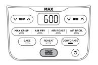
6 When dehydrating is complete, the unit will beep and END will appear on the control panel display.
